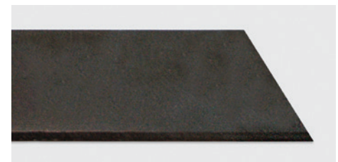
Powercron AdvantEdge Electrocoat: <5 Rust Spots
